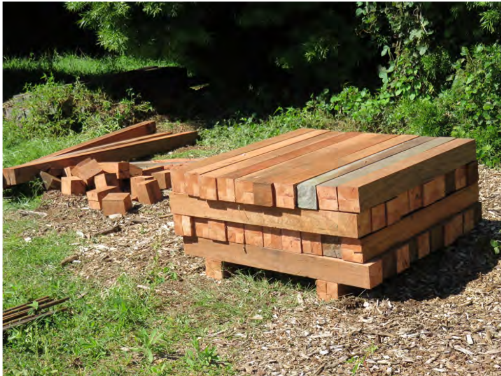
42 inch steps cut from 7 foot 4X4 Eucalyptus posts, supplied by South Pacific Lumber, are ready for project weekend. Each post weighs approximately 40- 45 pounds.
